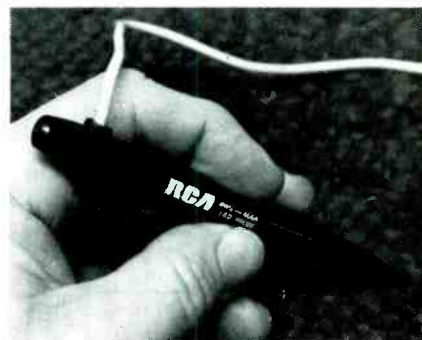
Fig. 8 A red LED in the end of the continuity probe lights to show resistances of less than about 5K ohms.
